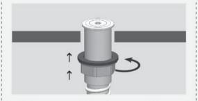
If you are using the soap tank support fix it to the desired location.
